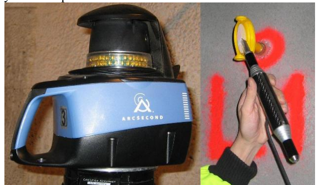
Figure 3: iGPS transmitter and sensor during a test in a tunnel
