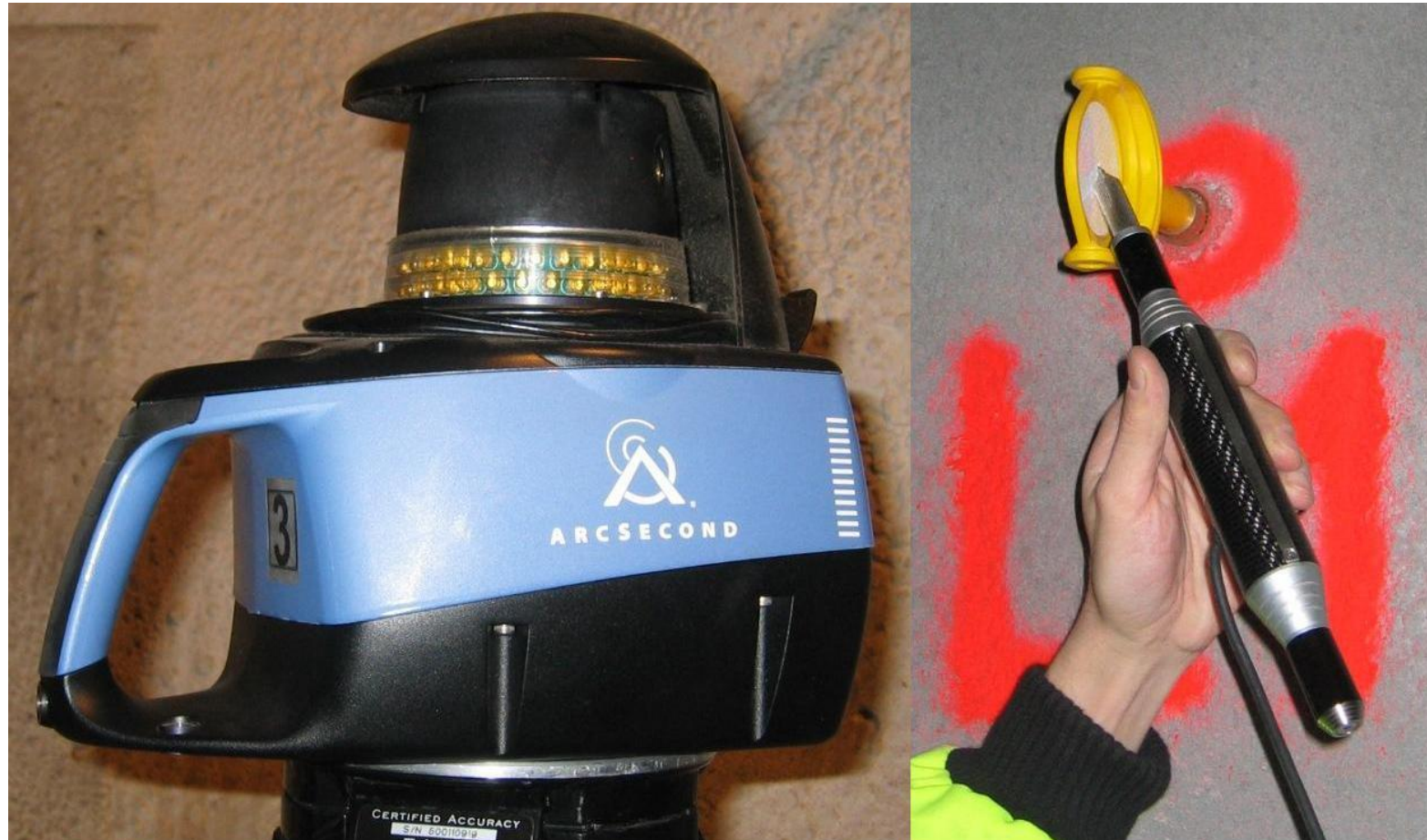
iGPS transmitter and sensor during a test in a tunnel
