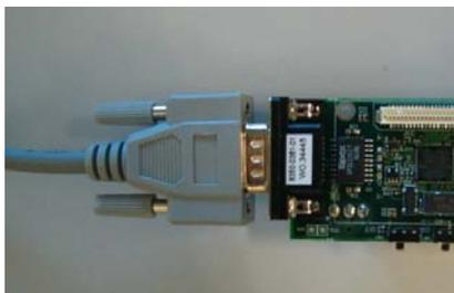
Figure 6: Cricket unit / RS232 cable assembly
