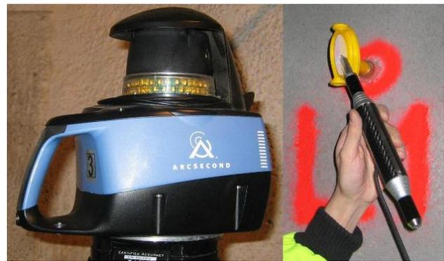
Figure 5: iGPS transmitter and sensor during a test in a tunnel
