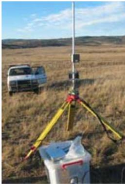
Figure 2: Locata antenna (Barnes et al. 2005)
